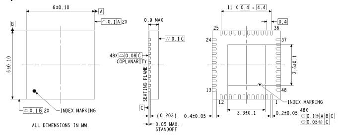
Figure 1. 48-lead sawn QFN, 6mm x 6mm Package Dimensions
