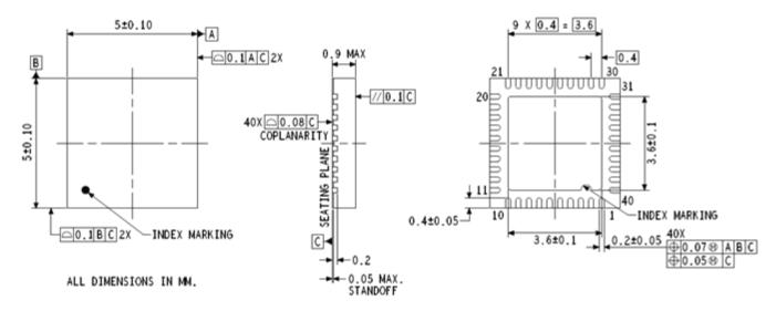
Figure 2. 40-lead sawn QFN, 5mm x 5mm Package Dimensions
