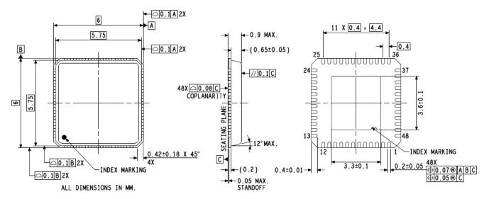
Figure 3. 48-lead punched sawn QFN, 6mm x 6mm Package Dimensions
