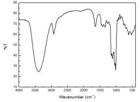
Fig. 2. FTIR characteristics peaks of the EPS produced by *L. fermentum* X1 (EPS in KBr tablet).
