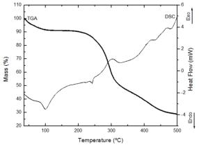
**Fig.1.**Thermogravimetric analysis (TGA) and differential scanning calorimetry (DSC) of the EPS from *L. fermentum* X1.
