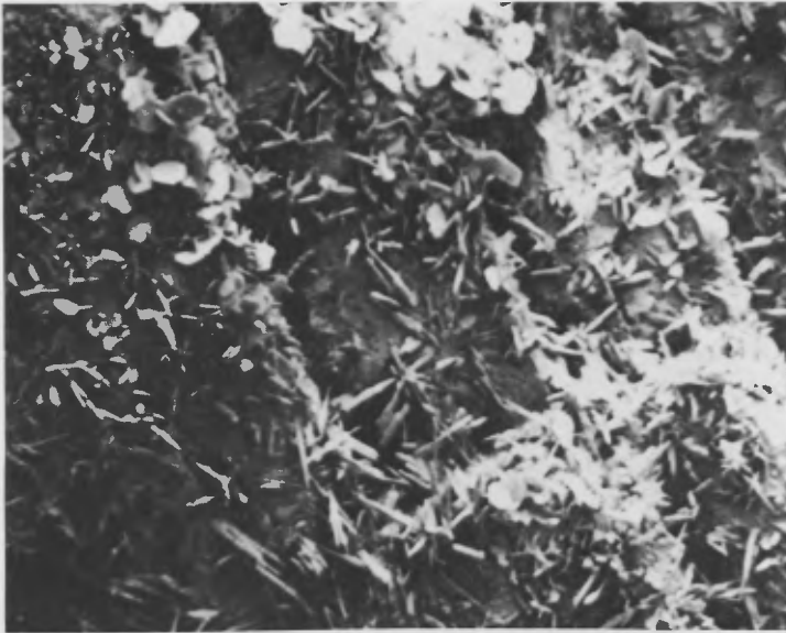
Fig. 7. Scanning electron micrograph of the oxidized galena ore. The spikey crystals are phosgenite ( \text{PbCl}(\text{CO}_3)_{0.5} ) and the plate-like crystals are hydrocerussite, \text{Pb}_3(\text{OH})_2(\text{CO}_3)_2 which overly the present galena crystals. Full width of the photograph is 750\mu\text{m} .
