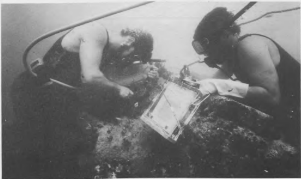
Fig. 4. Drs. MacLeod and North measuring corrosion potentials on the Xantho site during the predisturbance survey. The concretion on a piston is being drilled so that the potential measurement on the underlying material can be made. Photo: Mike McCarthy.
