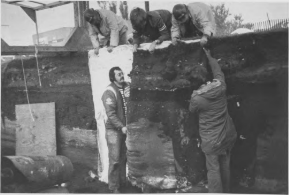
Figure 2. Peeling of the transfer from the soil profile.
