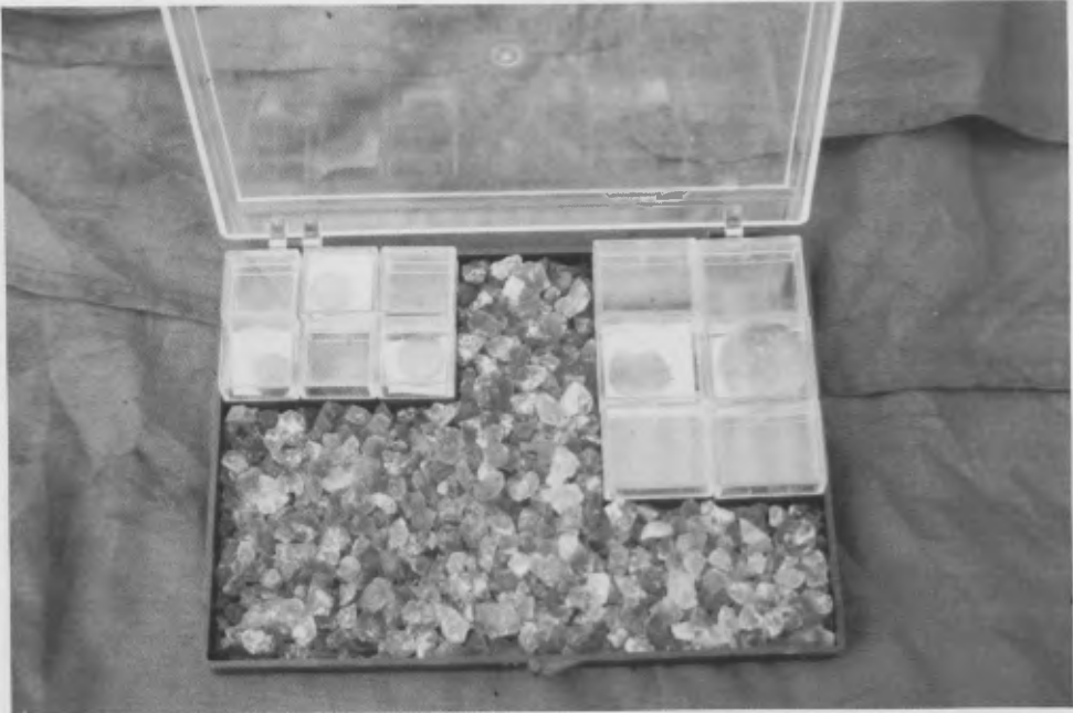
Figures 7-8. Coins were enclosed singly with silica gel inside small containers with transparent closures and glued shut; the small boxes were then placed in similar, but larger, containers, with silica gel and an air-tight seal. Photo: author.
