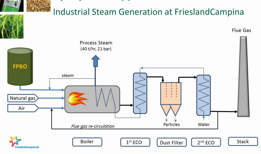
Schematic drawing of Process Steam Boiler at FrieslandCampina
