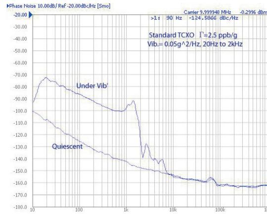
and then observing the effect on the output spectrum. When the applied vibration is a single frequency sine wave, a discrete spur will be produced offset from the carrier by the vibration frequency. By measuring the level of this spur relative to the power of the carrier, the amount of frequency devi-
