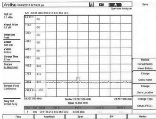
Figure 3.1-3 (T) Spectrum Photos 28 GHz - 100 kHz Res BW Site 10 at 2m AGL
