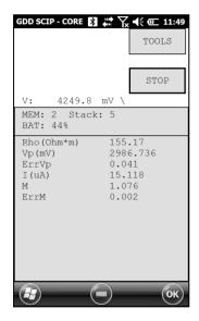
In constant current mode, if a little red square appears in the window that means that the signal is saturated. Stop the measuring process, select a lower current and start the readings over. These instructions appear in a pop-up window when you click on the red square.
