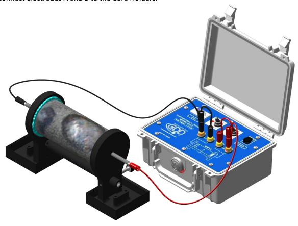
8. During the whole measurement process, the surface between the core holders should always be completely dry.
