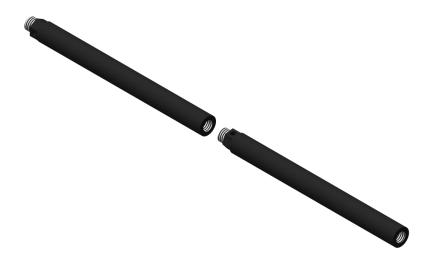
The rod fixes the two holders together. Move one of the holders along the rod to keep the core sample in place. It is possible to connect two or three rods together if the core sample is too long for one rod. To affix the rod, insert and screw. To remove the rod from the holder, unscrew the rod. If it becomes hard to unscrew the rod, use a 5/8" wrench or the Allen key provided with the Core Holder.
