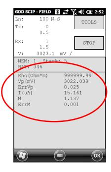
6. To take a second reading click on START. The following window appears. Then click on INC and the station will increase by the displacement increment. Click OK and the reading process will start.
