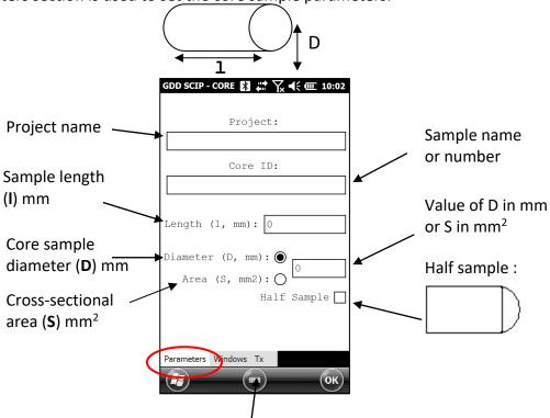
Open the keyboard at the bottom of the screen by clicking on it. You can also use the numeric keypad of the Archer<sup>2</sup> Field PC to enter numeric values. Use the tab key to advance the cursor to the next tab stop.
