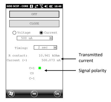
You cannot change the value of the transmitted voltage or transmitted current while the transmitter transmits.
