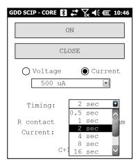
Click on the ON button to turn the transmitter on. The transmitted current appears. The little green square indicates the transmitted signal polarity.
