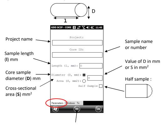
Open the soft keyboard at the bottom of the screen by clicking on it. You can also use the numeric keypad of the Archer2 Field PC to enter numeric values. Use the tab button ( ) to advance the cursor to the next tab stop.
