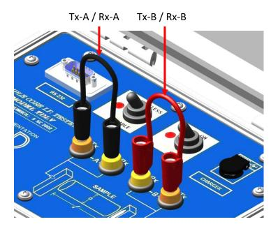
7. Connect electrodes A and B to the Core Holders.
