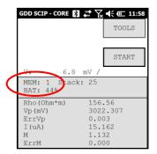
19. Click on 'Tools' and select 'Memory' to create a file with your saved data (or press → 1, and ← on the keypad to open the Tools menu and press shift ① + 8 ▼ or 2 ▲ to highlight the different options). Click on 'Save File' (or press ← when Save File is highlighted).
