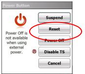
If the Power Button menu does not appear, hold the On/Off key for a full count of 20 seconds (*Hard Reset*) even through the blue screen with sliders, if it appears.
