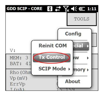
Select Voltage if you need a constant voltage, or Current if you need a constant current. The contact resistance appears automatically.
