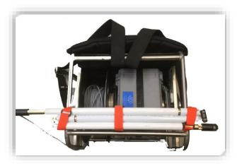
The borehole SCIP probe is very useful for detail IP surveys in drill holes. The probe can be used in Dipole-Dipole or Wenner configuration according to the electrode connections.
