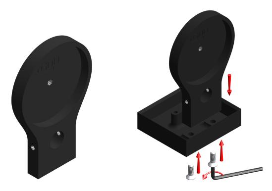
The two holders keep the core sample in place. Fix the holders to the receptacles with two bolts using the Allen key provided with the Core Holder.
