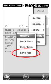
20. When this screen appears, the GDD *Generic* file option will be selected by default (.gdd file). The *Geosoft* option can be chosen to create a specific file to be imported in *Geosoft* software. Take note that in the *Geosoft* file (.dat file), some information as core ID, length and diameter is missing. The *Fullwave* option can be selected to create a file that contains the full waveform sampled data.
