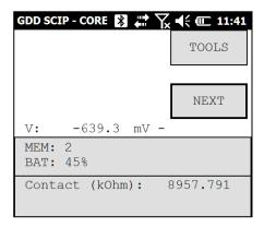
If the value of the core resistance is higher than 50 000 kOhms (50 MOhms), the value of the chargeability could be affected. If this should be the case, if you click on NEXT, the following message should appear:
