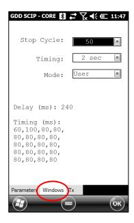
The time to get one reading increases with the number of stacks and the signal timing. It could take up to three (3) hours to get one reading with 50 stacks at a timing of 128 seconds.
