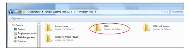
10. Use the drag and drop or the copy and paste functions to move the new GDD SCIP software files from your computer to your Archer<sup>2</sup> PDA's new GDD folder.
