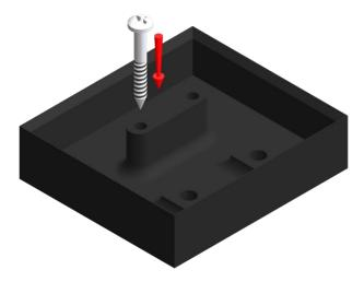
The two receptacles must be used to keep the surface between the two core holders dry. The receptacles keep all the liquid (water, copper sulphate) in them. It is possible to screw the receptacles onto a table using the two base holes.
