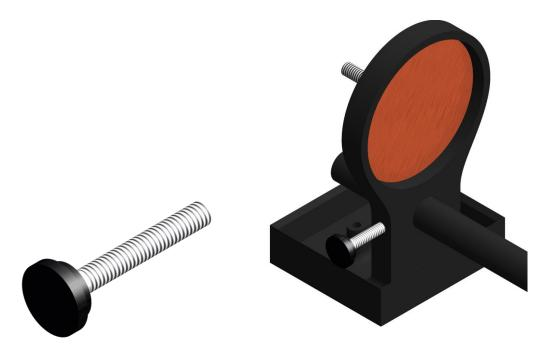
The fixing screw holds the holder in place along the rod.
