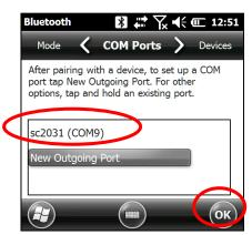
16. The name of your SCIP tester should appear with the *COM9* tag. Click on the *Ok* button to close the window.
