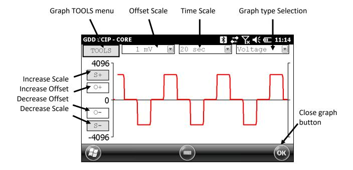
1. Select offset scale. The offset is in mV for the Voltage graph and in uA for the Current graph.
