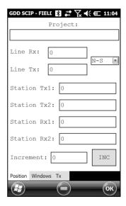
Enter a line number and select the line direction. A negative number cannot be entered for the line; the labels N, S, E and W are used to define the direction.
