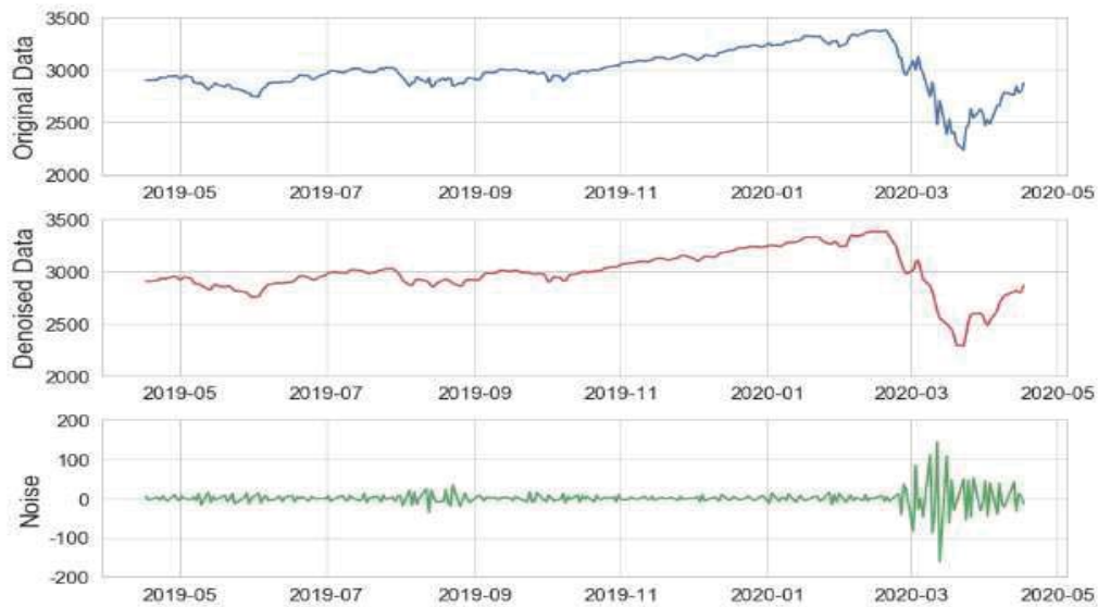
Figure 20. The sample of data before and after performing the P-FTD and the noise removed [5]
