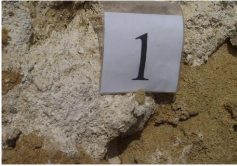
Fig. 6 - PSC-M1 sample – bedding mortar. The mortar is easy to breakage, whitish in color and full of shells inside.
