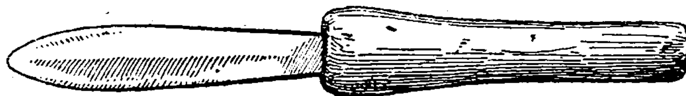
FIG. 14 (scale \frac{1}{4} ). Kesimoret , knife used for tapping palms.
