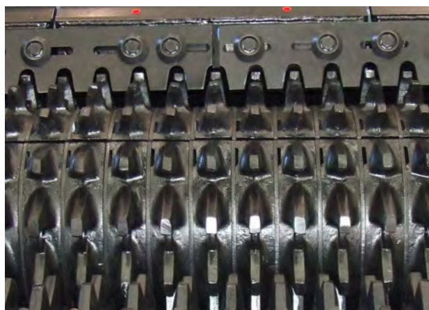
Integrated scraper system
