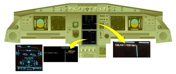
Figure 2. ECAM FC CTL system page, ECAM status page, ECAM Engine/Warning display on the event of ELAC 1 PITCH FAULT
