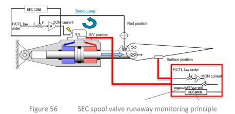
For SEC spool valve monitoring, a trend monitoring principle is used (rather than position monitoring), which can detect erroneous control surface movement (e.g. surface movement in the opposite direction of the given order). If a spool valve runaway signal is detected, a centering command is launched, and the control is released to the next computer.
