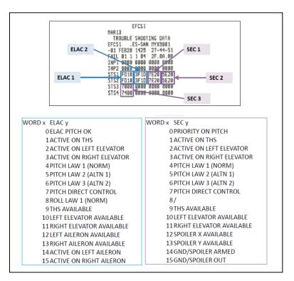
Figure 39 TSD decoding and information stored.
