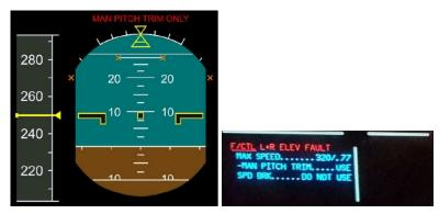
Figure 17 PFD display in PITCH mechanical back-up, ECAM procedures displayed in mechanical backup.
