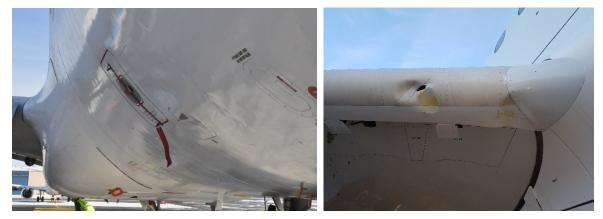
Figure 31 A/C skin wrinkled, fairings damaged by landing lights; slat punctured
