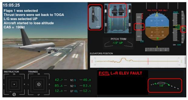
Figure 6. Cockpit inputs and indications at 15:05:25
