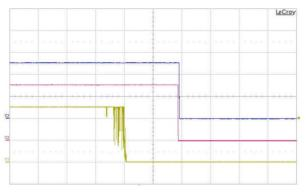
Figure 52 While ground setting is launched and manual input is held, switch 1 signal is activating with abnormal spikes. Switch 2 and 3 appears with delays after 2s.
