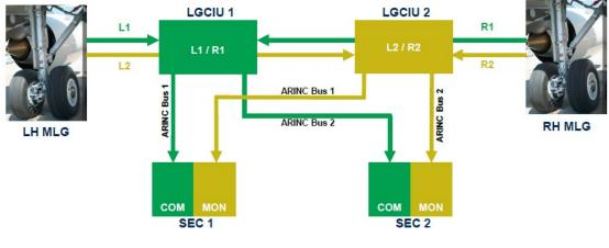
Figure 57 LGCIU-SEC communication architecture
