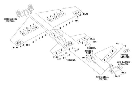
Figure 23 Actuation of flight control surfaces
