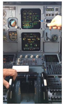
Figure 42 Actuation of the pitch trim wheel
