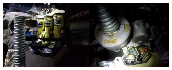
Figure 43 Camera recording the PTA micro-switch movement
