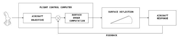
Figure 15 Basic principle of control laws
