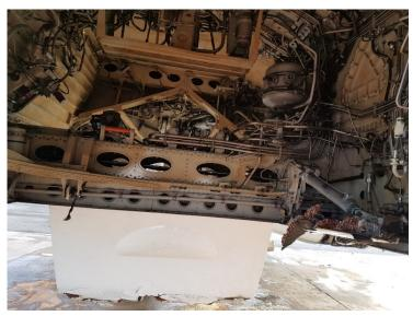
Figure 35 RH landing gear actuator and missing door
