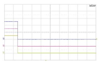
Figure 54 Nominal signals from all 3 switches while ground setting is launched and manual input is held
