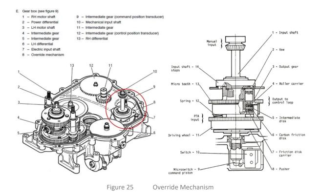
When the crew touches the trim wheel, torque is applied on the mechanical input shaft (Figure 25, item 1). If the applied torque is greater than or reverse of the PTA input (from the electrical motors), the roller carrier and roller (4) will disengage from the vee (2), push the roller carrier and friction disk
