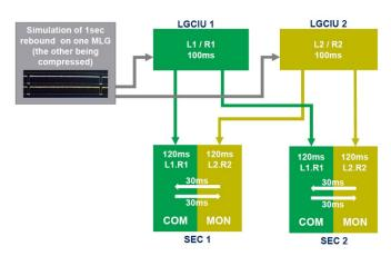
Figure 62 Simulation setup for MLG 1s rebound test
