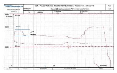
Figure 55 Override test results, the actual friction curve is slightly under the required criteria
