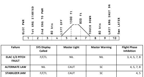
Figure 22 Alert inhibition in flight phases
