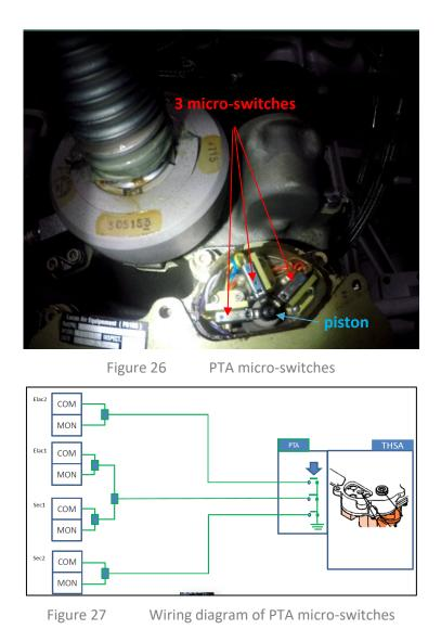
When Auto Trim is active the commanded stabilizer position is measured by the COM transducer. A reduction gear assembly in the THSA transfers the commanded stabilizer position to the COM transducer (Figure 25). A separate MON transducer measures the actual stabilizer ball screw position. The ELACs and SECs monitor both COM and MON transducers and if there is a discrepancy in the measured results fault message will be generated.
