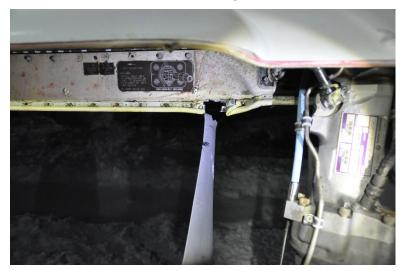
Figure 37 Damaged RAT blade tips and rat doors
