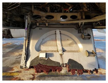
Figure 34 Bent LH landing gear actuator and damaged door
