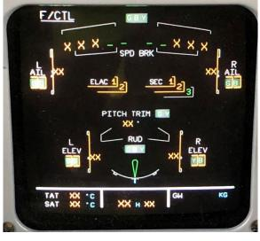
Figure 20 ECAM F/CTL page with SEC 3 active
