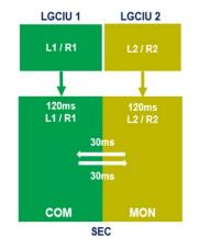
Figure 59 SEC logic is used to consolidate the ground or flight mode
