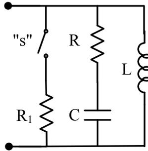
Datos:  $R = 10\Omega$        $R_1 = 20\Omega$        $C = 10\mu F$        $L = 2mH$
