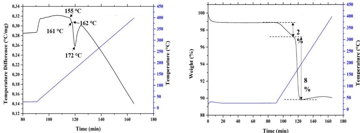
Figure 14: DTA-TGA plots of a sample of  $\alpha\text{-AlH}_3$  before treatment
