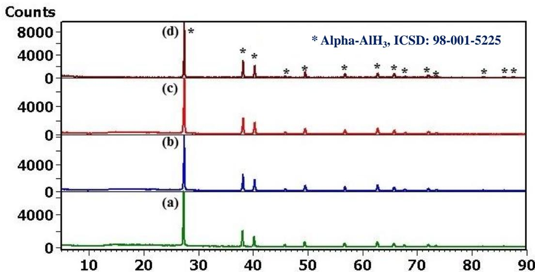
Figure 9: XRD patterns of synthesized alane: (a) not washed, (b) washed with 15 %, (c) 10 % and (d) 5 % HCl
