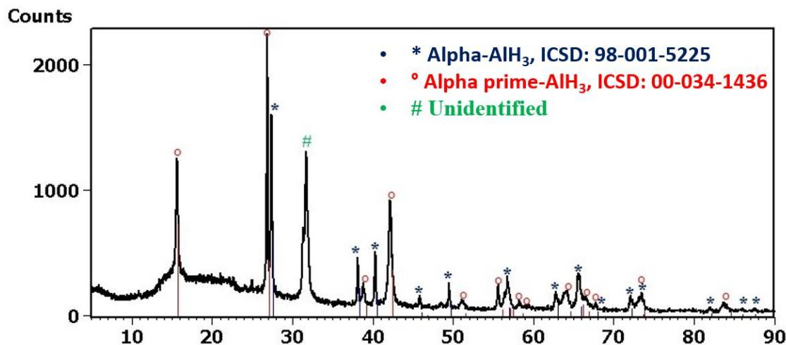
Figure 12: XRD pattern of alane after “recrystallization”
