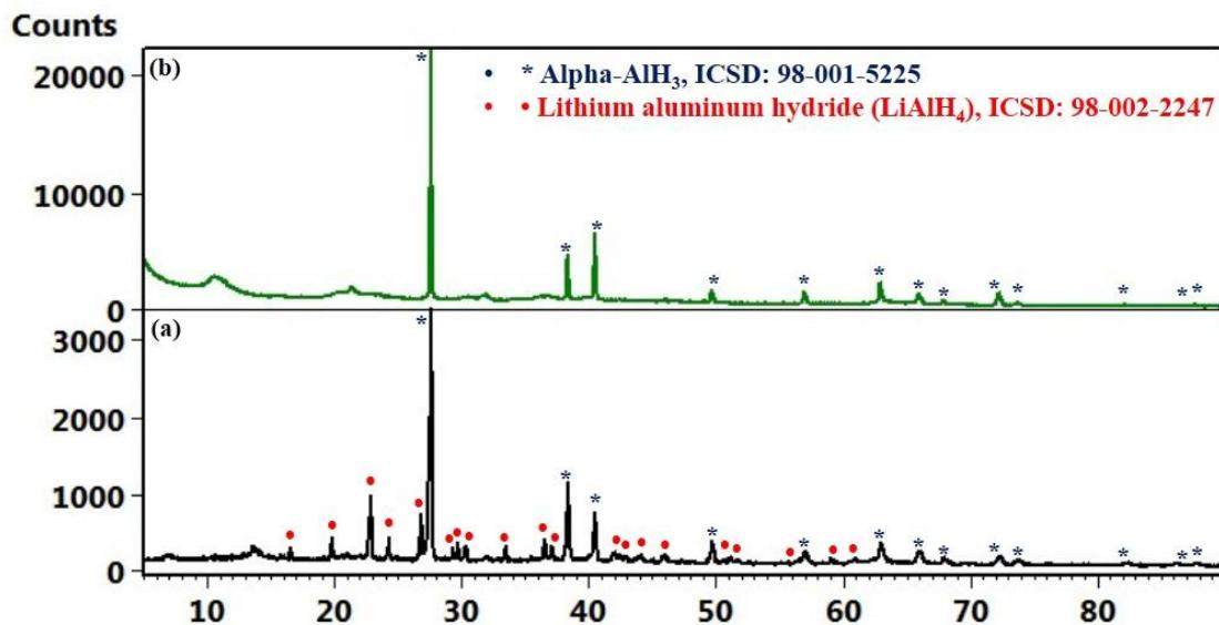
Figure 7: XRD pattern of synthesized AlH<sub>3</sub>: (a) before washing with THF, (b) after washing with THF
