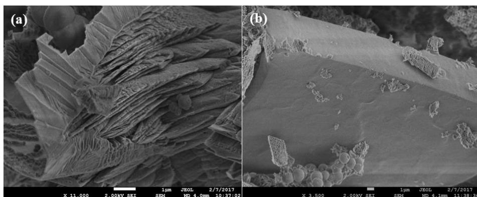
Figure 11: SEM images of a sample of AlH<sub>3</sub> before (a) and after (b) washing with 15 % HCl. Scale bars at the bottom of each photograph represent 1  $\mu$ m
