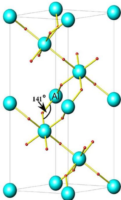
Figure 1: Interconnection of the  $\text{AlH}_6$  octahedra in the structure of  $\alpha\text{-AlH}_3$  composed of Al–H–Al bridging bonds with an angle of  $141^\circ$  [10]
