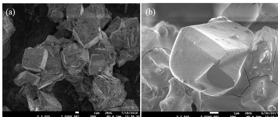
Figure 10: SEM images of a sample of AlH<sub>3</sub> before (a) and after (b) washing with 5 % HCl. Scale bars at the bottom of each photograph represent 1  $\mu$ m
