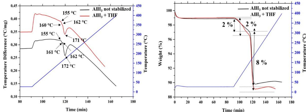
Figure 16: DTA-TGA plots of a sample of  $\alpha\text{-AlH}_3$  before and after been stabilized by THF
