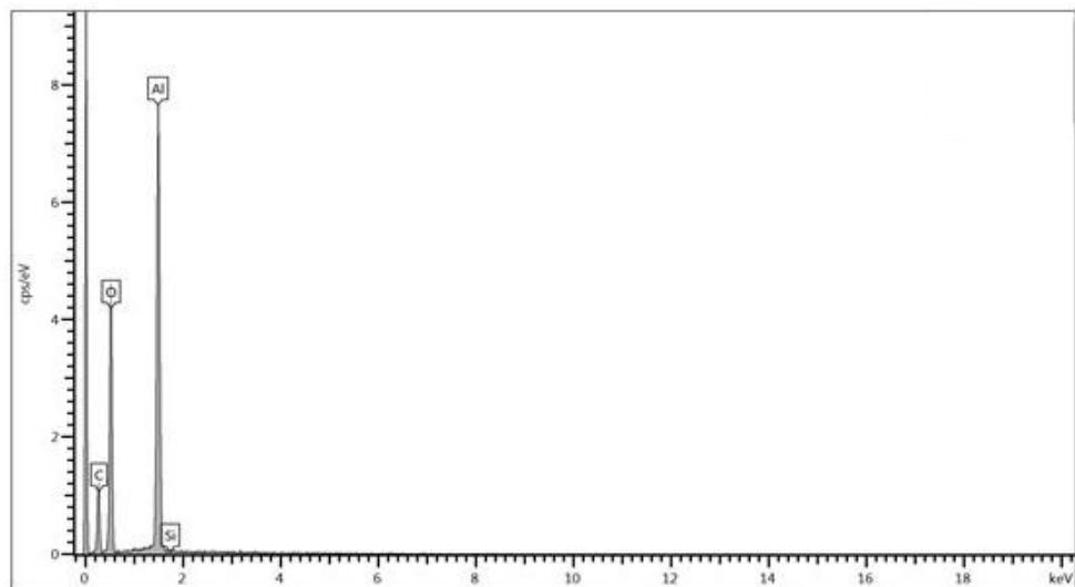
Figure 5: Elemental composition of spherical particles performed by EDS
