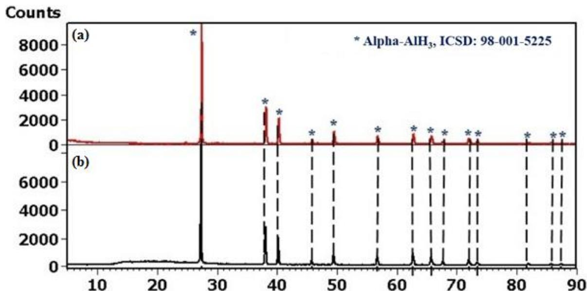
Figure 2: XRD patterns of synthesized α-AlH<sub>3</sub>: (a) 12 g of α-AlH<sub>3</sub> batch, (b) 6 g of α-AlH<sub>3</sub> batch
