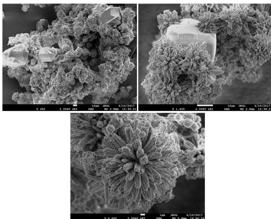
Figure 13: SEM images of a sample of AlH<sub>3</sub> obtained after “recrystallization”. Scale bars at the bottom of each photograph represent 10  $\mu\text{m}$  for photographs on top, 1  $\mu\text{m}$  for the one at the bottom
