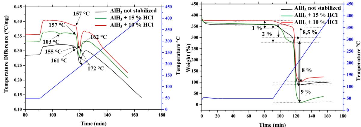
Figure 17: DTA-TGA plots of a sample of  $\alpha\text{-AlH}_3$  before and after washing with 10 % and 15 % HCl
