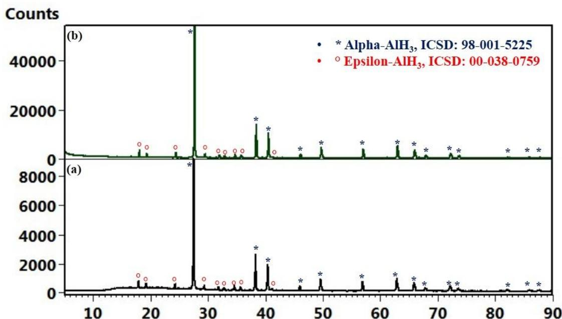
Figure 6: XRD pattern of synthesized AlH<sub>3</sub>: (a) before washing with THF, (b) after washing with THF
