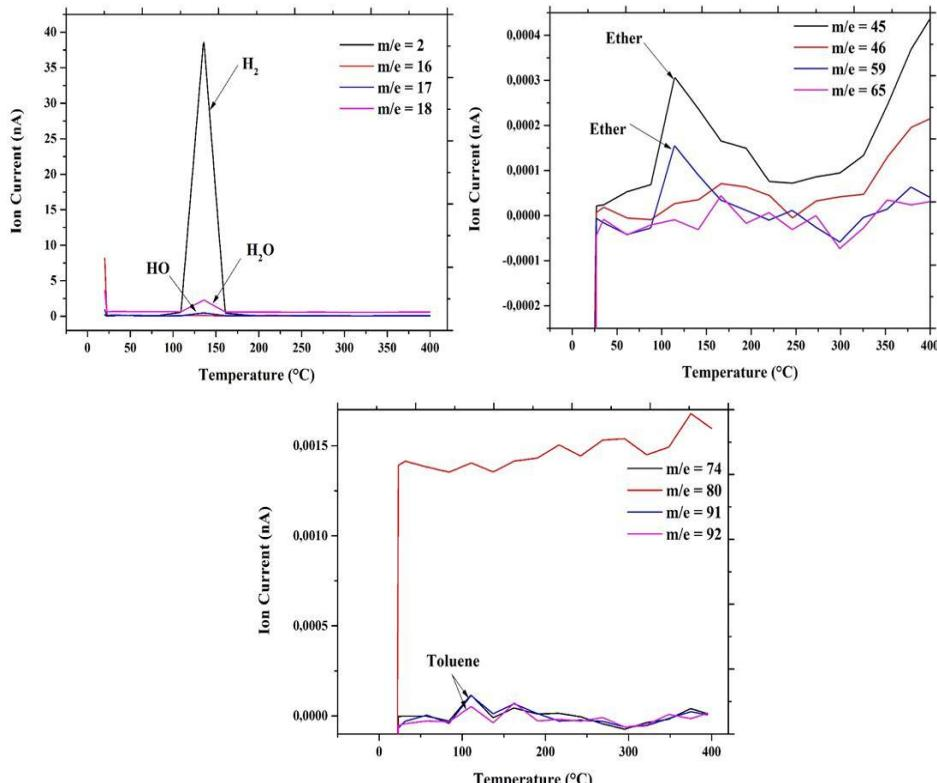
Figure 15: Mass spectroscopy (MS) of a sample of  $\alpha\text{-AlH}_3$
