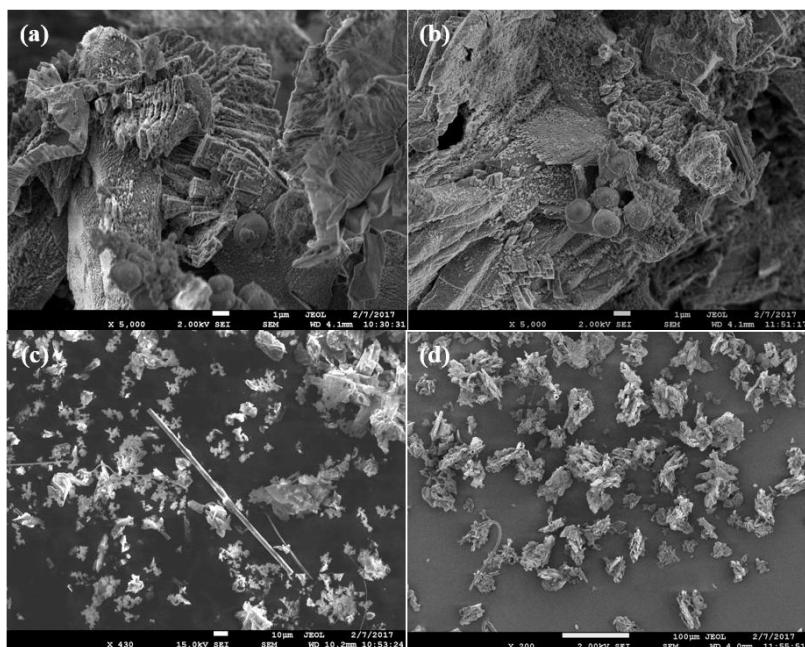
Figure 8: SEM images of a sample of AlH<sub>3</sub> before (a and c) and after washing with THF (b and d). Scale bars at the bottom of each photograph represent 1 μm for a and b, 10 μm for c, 100 μm for d
