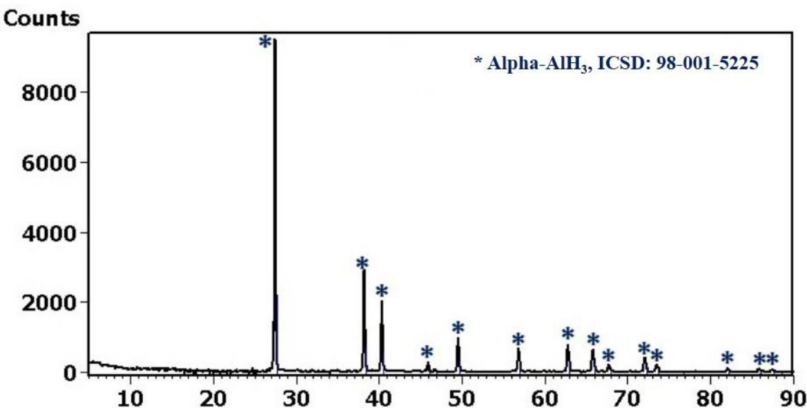
Figure 3: XRD pattern of synthesized  $\alpha$ -AlH<sub>3</sub> before stabilization tests
