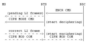
If the TRX for some reason can not perform the enciphering as requested in the ENCRYPTION COMMAND, the TRX shall return an ERROR REPORT message, e.g., with the cause "Encryption algorithm not implemented".
