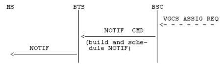
If the BTS for some reason can not perform the notification commanded by the BSC, then the BTS shall return an ERROR REPORT message with the relevant cause value.
