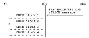
With the SMS BROADCAST COMMAND mode of operation, the BSC can also set the BTS broadcast default mode. The BTS is then responsible for transmission of a default message when no other message is to be broadcast.
