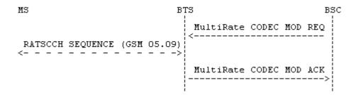
If for any reason, the BTS is not able to complete the MultiRate Codec Configuration change, it should send a MultiRate CODEC MOD Negative ACK with the most appropriate cause.
