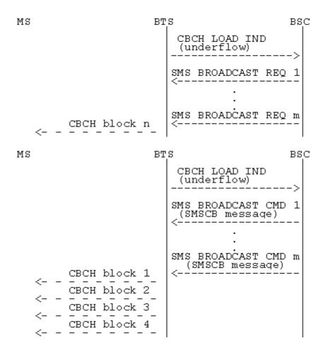
With the CBCH LOAD INDICATION mode of operation, the BTS can also request immediate stop of broadcast for a period of m (=amount indicated in the CBCH Load Information element) message slots in the overflow situation. BSC shall stop the broadcast for a period of m message slots and after that continue the broadcast of messages according to its own timetable.
