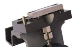
Photograph on left: Place the step block to one side, allowing the indicator tip to touch the flat zero reference surface of the step block. Photograph on right: Slide the step block to the other side to allow the indicator tip to extend into the step.
