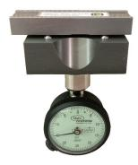
Step Block Reading with the 0.015 inch step block.
