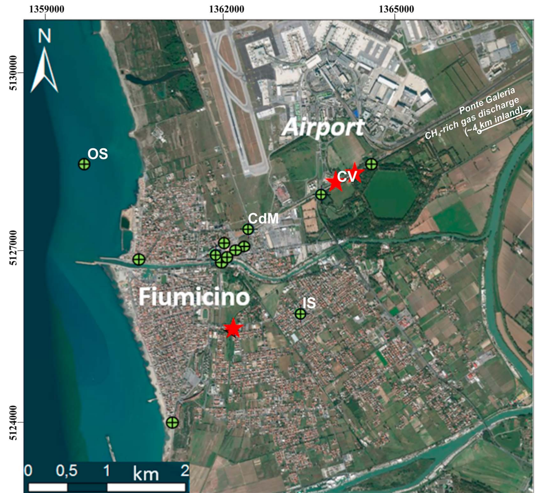
Figure 11. Fiumicino area with location of the gas discharges (red stars) and of blowout producing wells (green dots). CV = Canale Vignole; CdM = Coccia di Morto; IS = Isola Sacra; OS = offshore. Coordinates WGS 1984 Web Mercator (Auxiliary Sphere).
