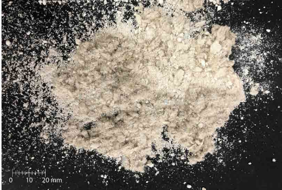
Figure 2a. Shredded drywall waste from demolition; Figure 2b: prototype DWB masonry.
