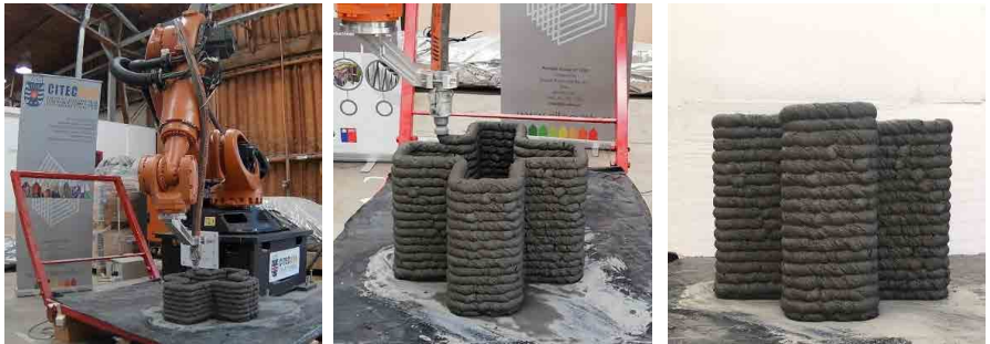
Figure 1. Printed construction experiments with a Kuka120 R2500 robot. Source (Authors 2020).
