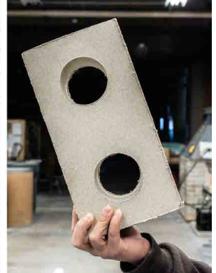
Figure 2a. Shredded drywall waste from demolition; Figure 2b: prototype DWB masonry.
