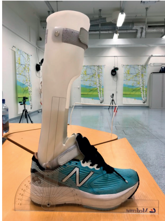
Figure 9. Example of bench alignment of a solid AFO with shoes; the shank/tibia inclined with a shank-to vertical angle of around 7°.
