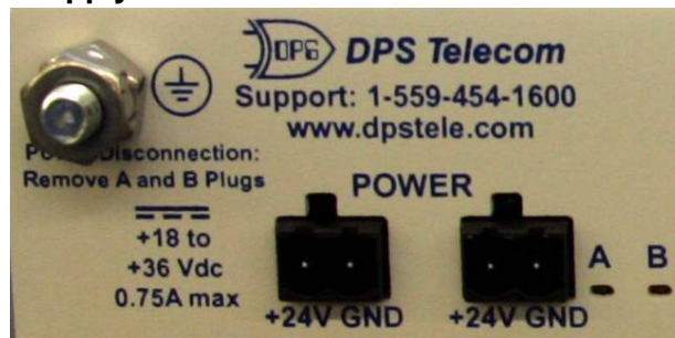
Grounding Lug left, dual power inputs right
