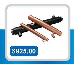
Nominal SLHE selections should be based on system horsepower, which will provide a nominal 10°F subcooling and a nominal 20°F suction superheat for R-22, R-502, R-404A, R-507, R-407A, R-504, R-134A, R-407C and R-410A at 110°F condensing and 25°F suction. For example, for a 1-1/2 HP system, select an SLHE 1-1/2. Do not select undersized models to avoid high suction pressure drops and gas whistling.
