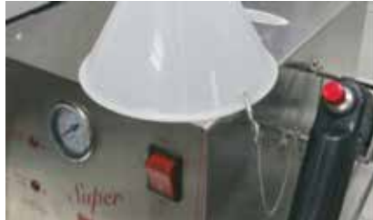
Figure 3: Funnel attached to the steamer to make it harder to make mistakes.
