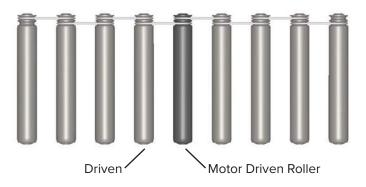
Double Groove Pulley Drive Layout:
