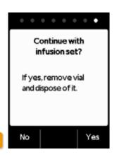
To proceed immediately with the connection of an infusion set, remove the vial and press Yes
