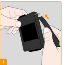
Pull both ends of the strap through the hook with each loop side facing outward.
