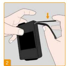
Secure the strap by pressing the hook side of the strap to the loop side of the strap.
