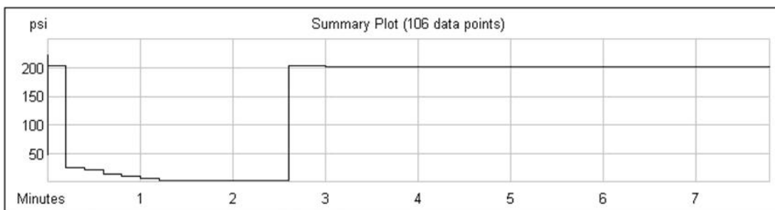
Figure 6-1 - Example of a Heat Fusion Joint Record (typical output for a McElroy Data logger)
