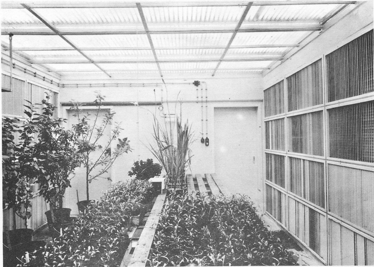
Fig. 3.- Part of a growth chamber. The air enters through the right wall and is evacuated through the left wall. The doors at the back give access to a dark room. In the future, plants will be grown on trolleys.
