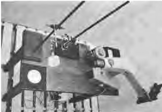
Fig. 2 .- Measuring apparatus. White circular plate : MgO film.
