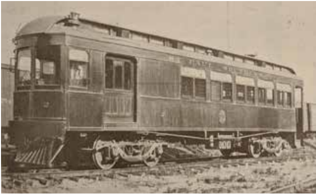
One of four cars used on the St. Paul Southern line. The electric cars ran on power from overhead lines, faintly visible in the photo (Guelcher, 227).
