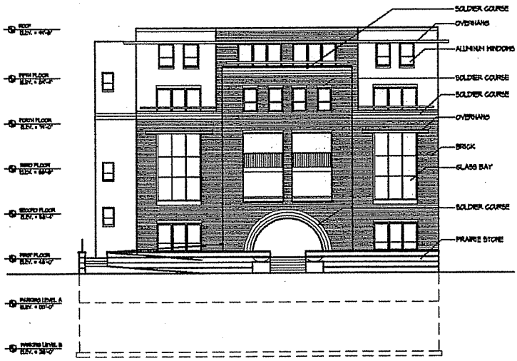
1 SOUTH ELEVATION SCALE 1/8" = 1'-0"
