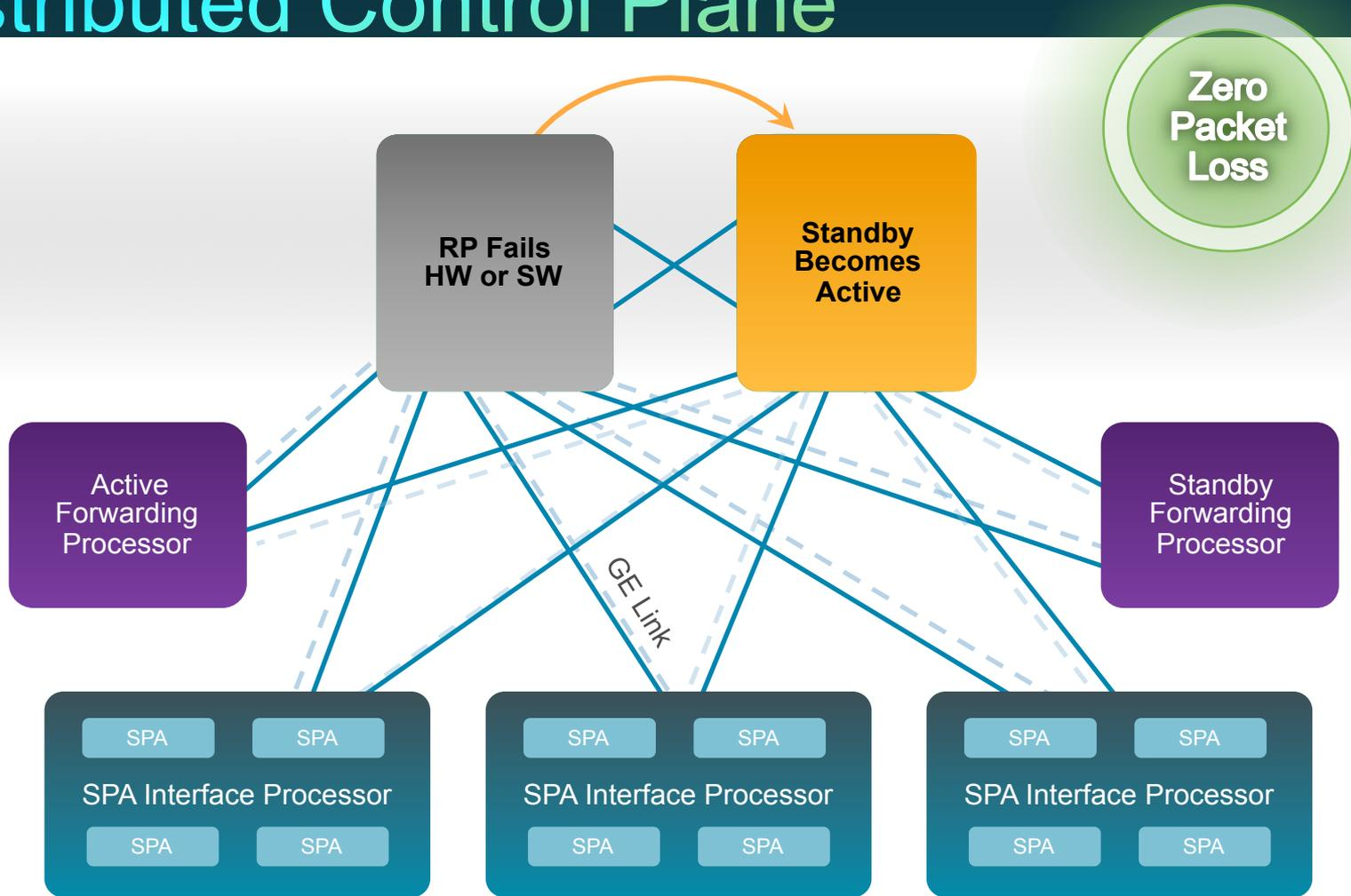
Separate and Independent Internal Communication Link for Control Plane (GE)
