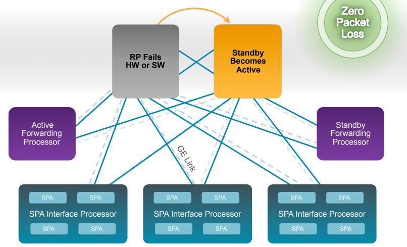
Separate and Independent Internal Communication Link for Control Plane (GE)
