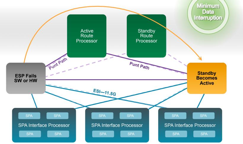
All Packets Processed by QFP for Forwarding Separate and Independent links for Data Plane communication (ESI 11.5G)
