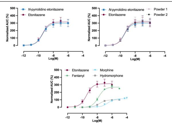
**Fig.3**  $\mu$ -Opioid receptor (MOR) activation profiles ( $n \ge 3$ ) obtained for *N*-pyrrolidino etonitazene and two independently sourced powders containing *N*-pyrrolidino etonitazene. Curves for morphine, fentanyl, etonitazene, and hydromorphone are shown for comparison. Data
