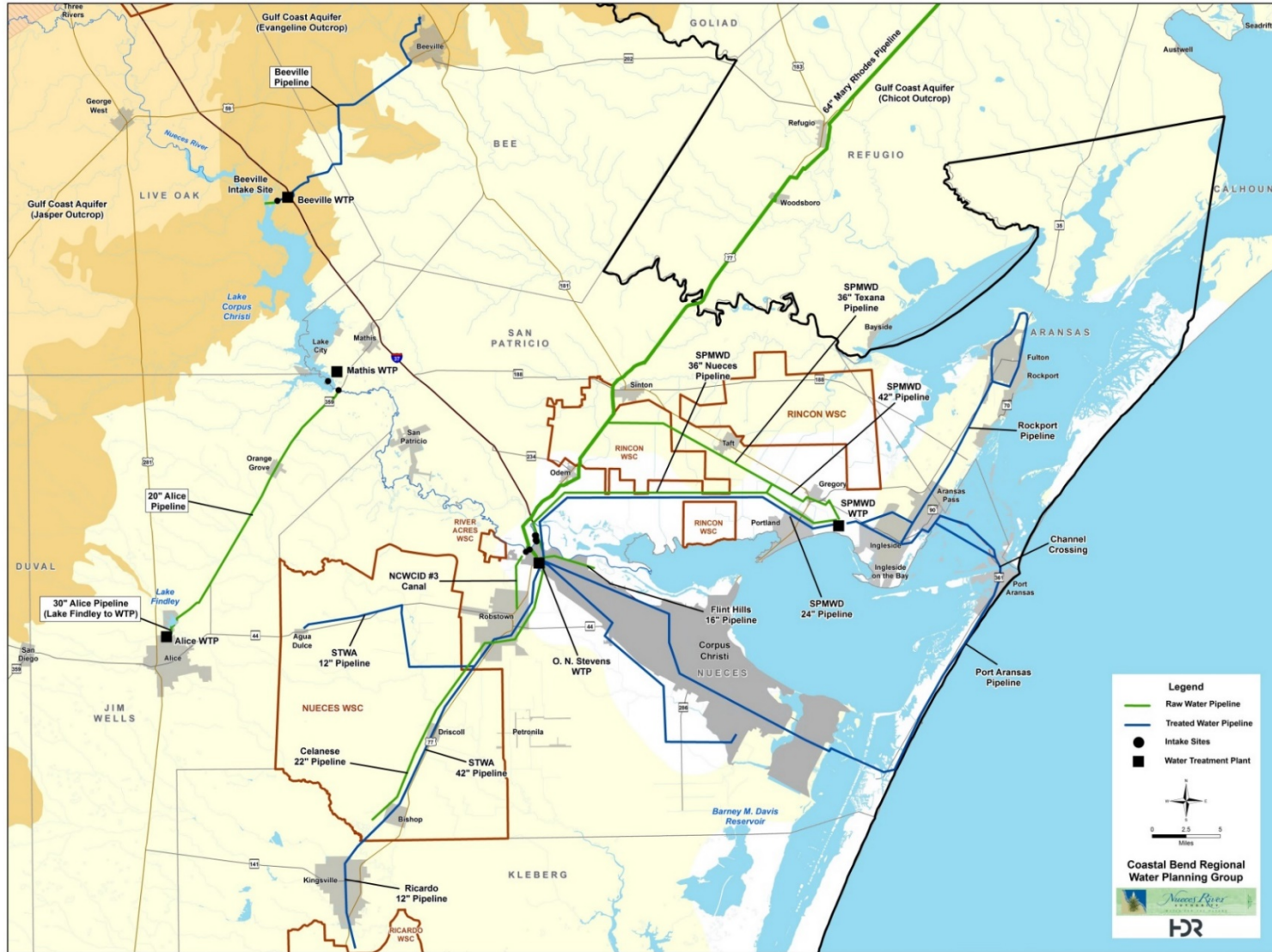
Figure 3.4. Coastal Bend Water Supply System
