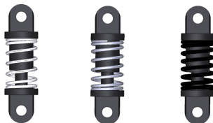
Figure 1-8. Low pressure springs (white; part number 9968-240) are included in the instrument spares kit. Use these springs if measuring delicate leaves that are damaged by the standard springs. Medium pressure springs (silver; part number 9968-131) are suitable for most leaves. High pressure springs (black; part number 9968-239) are used with the 6×6 cm chamber.
