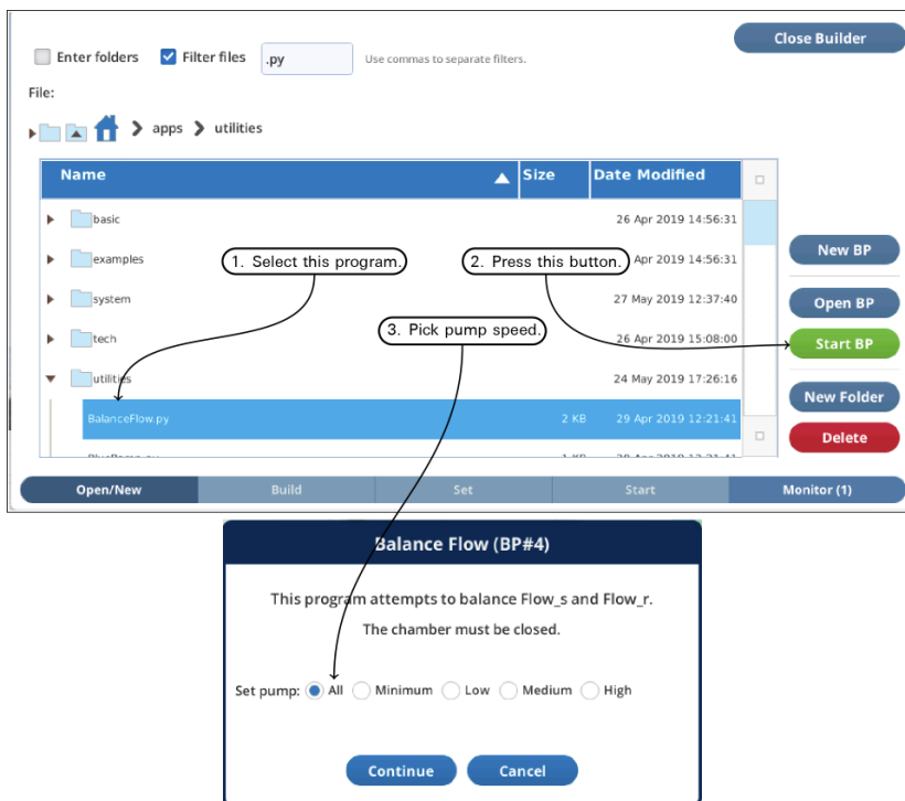
Figure 3-10. The BalanceFlow utility program can be run manually to determine (and automatically update) balanced flow set points.
