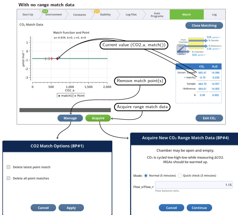
Figure 4-10. The CO 2 Match Data screen shows an expanded version of the CO 2 graph.
