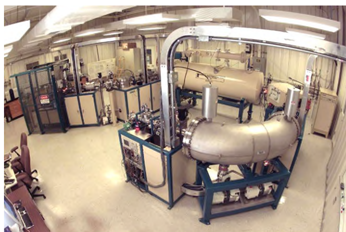
Figure 3. Accelerator mass spectrometer at the Lawrence Livermore National Laboratory in the USA. 5
