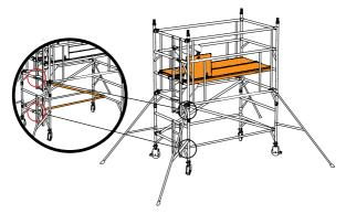
If clear access to the ladder is required, braces may be re-positioned as shown. Reposition braces to original location before moving tower.
