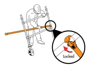
Position the second end frame as shown and fit the other end of the horizontal brace on to the vertical, just above the bottom rung. Fit a second horizontal brace on the bottom rungs on the other side of the frames to square the tower. Note: Check all brace claws are positively locked after fitting.
