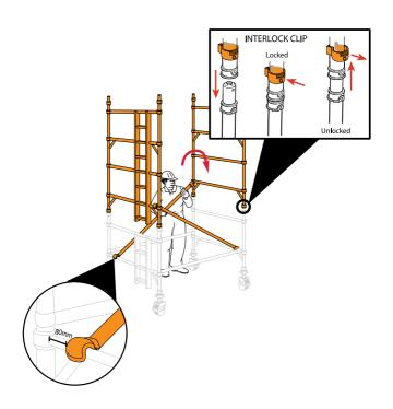
Fit a camlock AGR on each side of the tower. The bottom of the AGR must be fitted to the 3rd rung of the tower, as shown. The AGR should be placed up against the end frame verticals. Secure AGR frame by pulling the locking handle firmly down onto the lower horizontal tube of the AGR (locked position).
