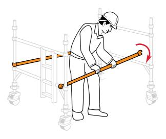
Fit two additional end frames ensuring ladder sections line up and check the frame interlock clips are engaged. Fit two diagonal braces (blue) in opposing directions, from the 1st rung to the 3rd rung on the opposing side. Diagonal braces should be positioned approx. 80mm inboard of the frame verticals. Ensure the frames are vertical and level by checking with a spirit level and setting the adjustable legs as required.
