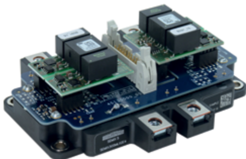
Figure 4: Single phase of SEMiX 5 3-Level Application Sample with two SKYPER 12 PV driver cores
