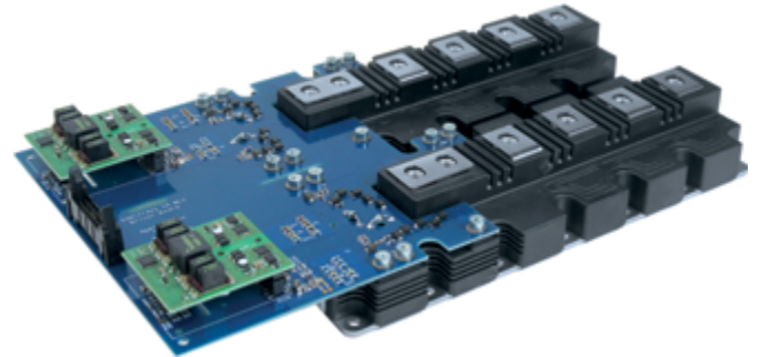
Figure 5: Single phase-leg of SEMITRANS 10 MLI modules with Application Board and SKYPER 42 LJ PV
