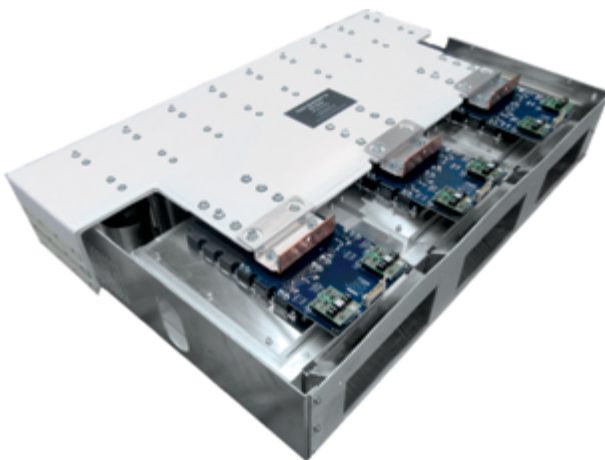
Figure 7: Three-phase, air-cooled power electronic stack based on SEMITRANS 10 capable of 1.25MW
