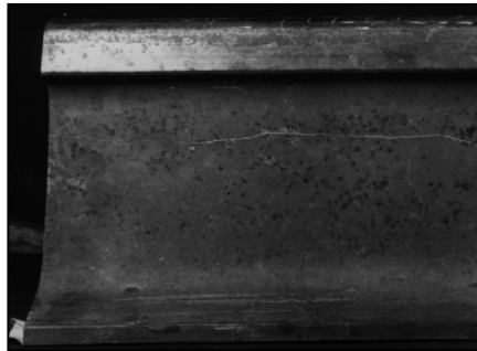
Section of Rail Containing a Split Web
