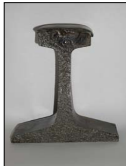
Engine Burn Fracture, Showing Small Transverse Separation
