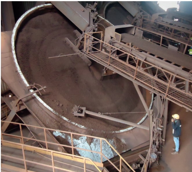
Fig. 3: Industrial scale pelletization process
