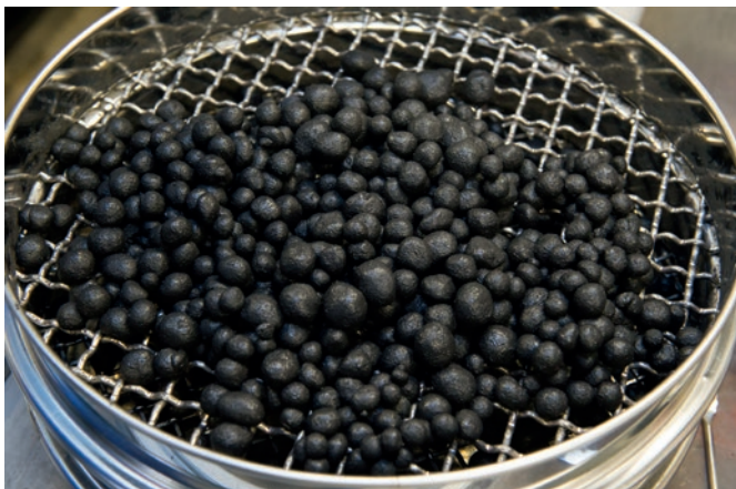
Fig. 4: Iron ore pellets produced from a magnetite ore in the lab
