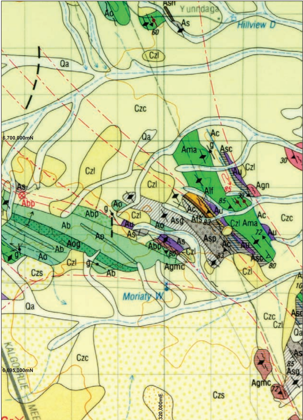
Figure 11.22: Moriarty Well area 1:25 000 scale study: Geological Survey of WA outcrop geology (part 'Menzies' 1:100 000 sheet, refer to Fig. 11.4b for legend). Grid is 1 km.
