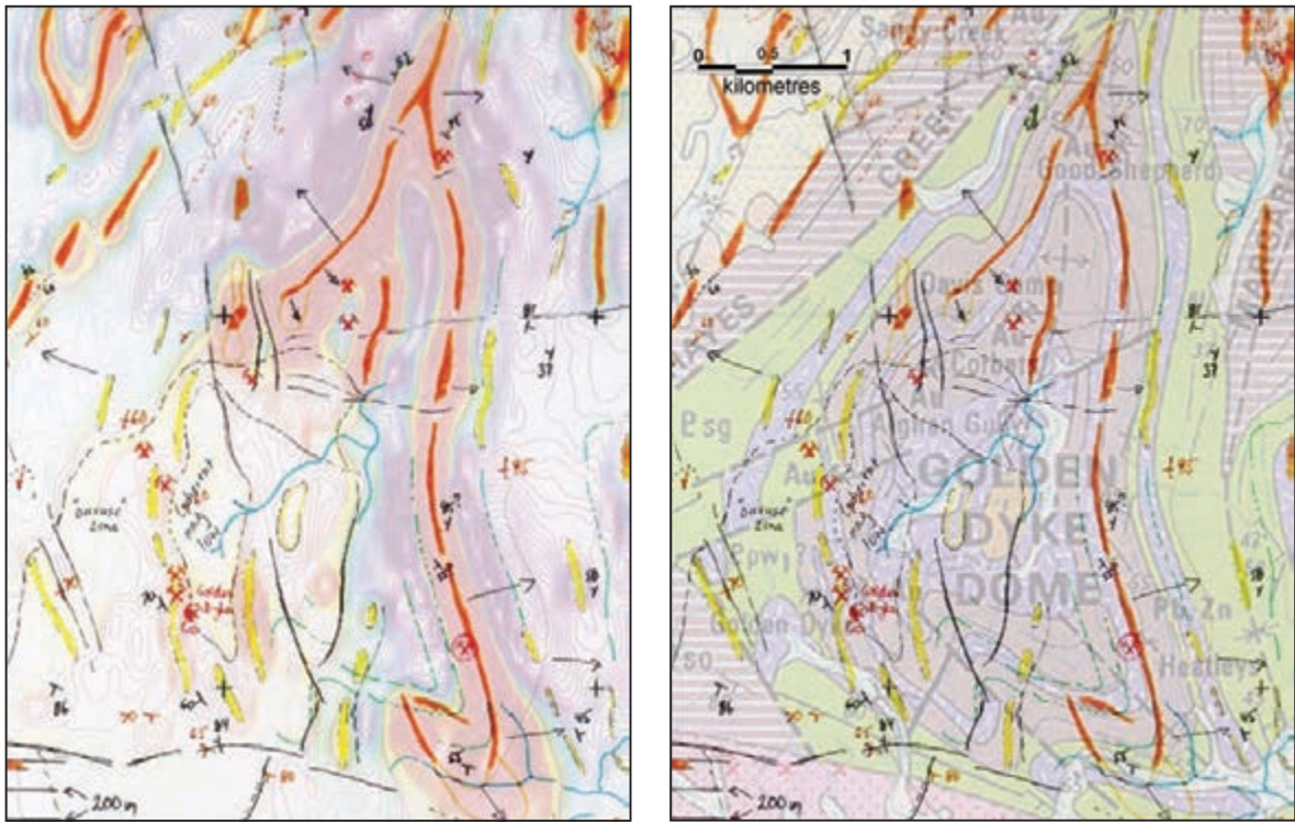
Figure 12.16a: Golden Dyke Dome – aeromagnetic observations on RTP 1st VD (left) and outcrop mapping (right). Refer to Figures 12.8, 12.12 and 12.14 for originals.
