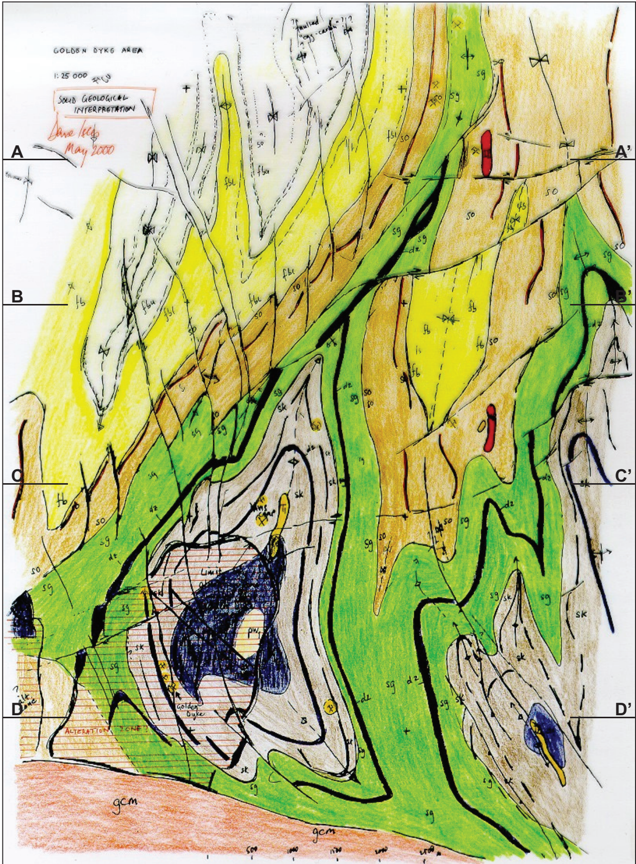
Figure 12.22: Working (draft) solid geology layer, showing cross-section locations. See Figure 12.20 for legend.
