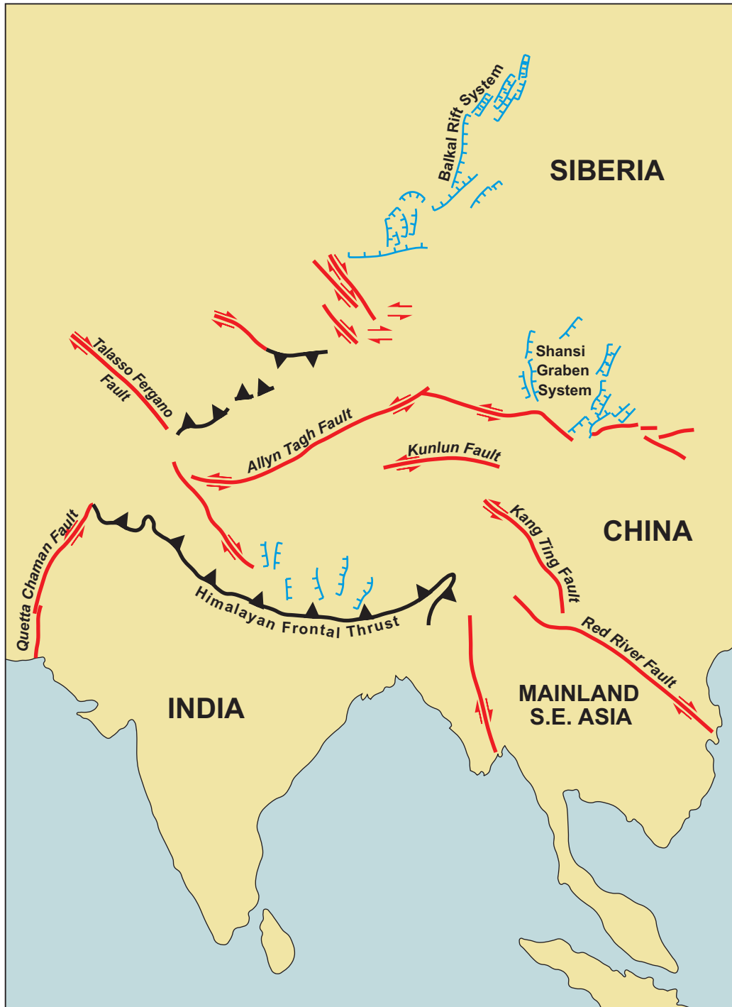
Figure 4.23: The extensive family of structures caused by the single progressive N-S deformation due to the impact of the Indian and Eurasian Plates (after Tapponnier et al. 1982). Compare this to the experimental deformation model in Figure 4.19.
