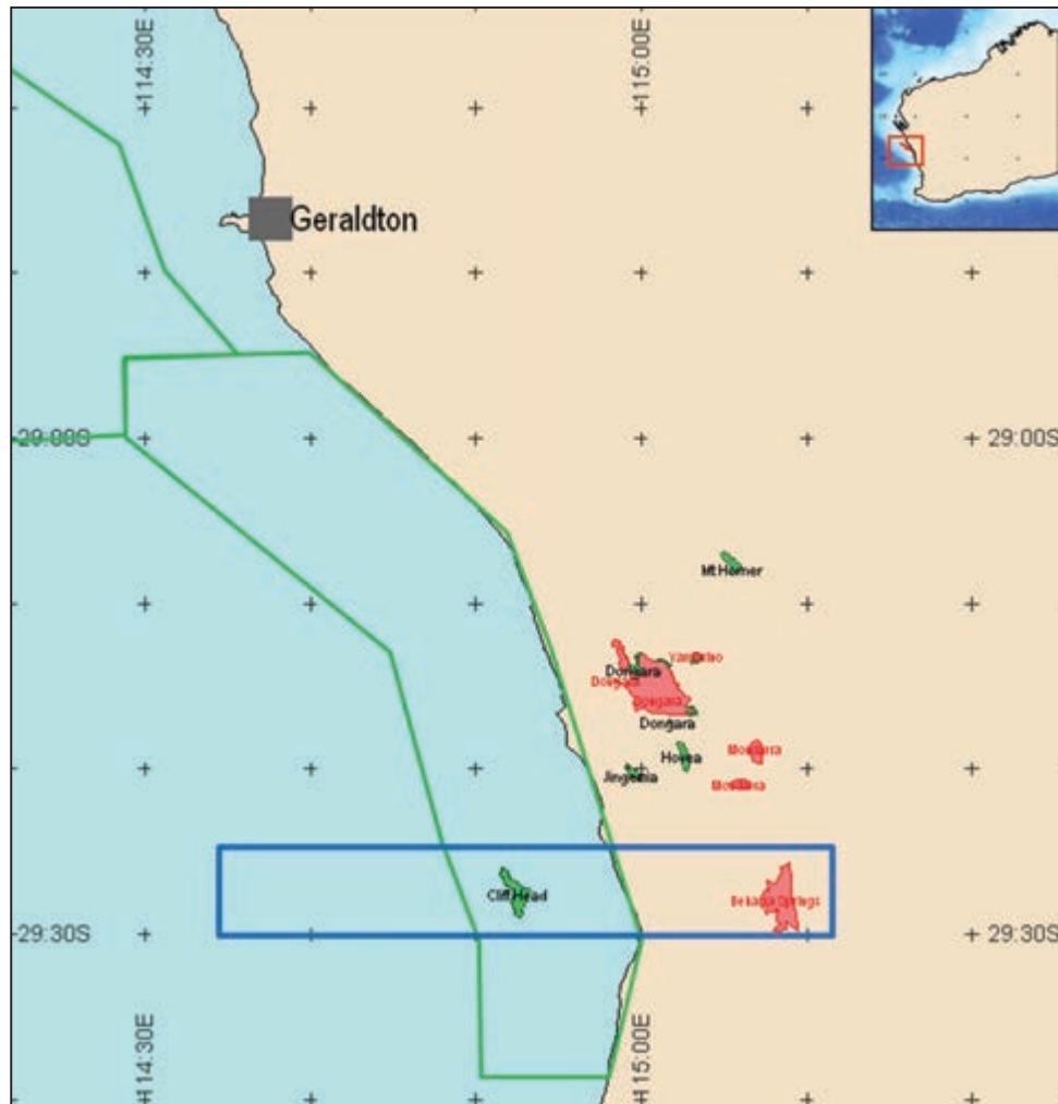
Figure 10.10: Location of Cliff Head Oil Field, ~15 km offshore and 80 km SSE of Geraldton. The blue box shows the outline of the aeromagnetic test strip acquired by Fugro Airborne Surveys in 2003 with a flight line spacing of 100 m. The green outlines show the more extensive aeromagnetic surveys subsequently acquired at 150 m line spacing by Roc Oil (WA) Pty Ltd as operators of the WA-286-P Joint Venture offshore WA.
