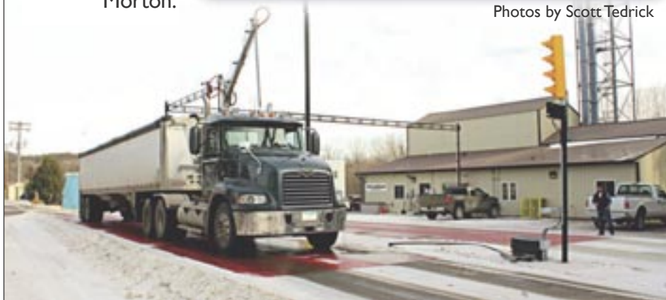
The Farmward Morton location added a new inbound and outbound scale this past summer to improve patron waiting and receiving times.
