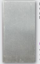
Panels pretreated with ACF-50 showed an average weight loss of only 1.9 mg.
