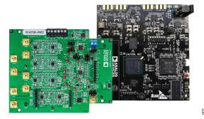
Figure 2. EVAL-AD7386-4FMCZ Board (Left) Connected to the EVAL-SDP-CH1Z Board (Right)
