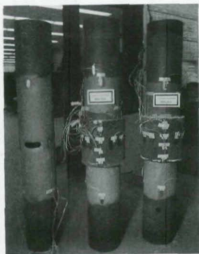
Fig. 20 Corrosion-Damaged Specimen 46-00-95, and Repaired Specimens 46-00-95-C and 46-00-95-E
