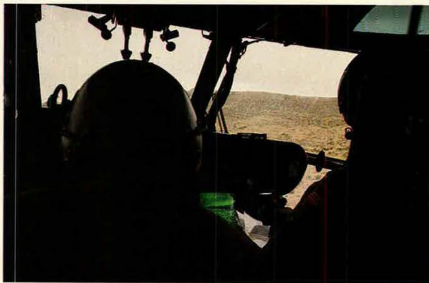
The MH-53J's forward-looking infrared system (green screen, center) enhances visibility for Maj. James Eustace (right), a pilot with the 1551st Flying Training Squadron, and MSgt. Arthur Burkett, flight engineer (left). The FLIR is especially important for low-level night flight.
