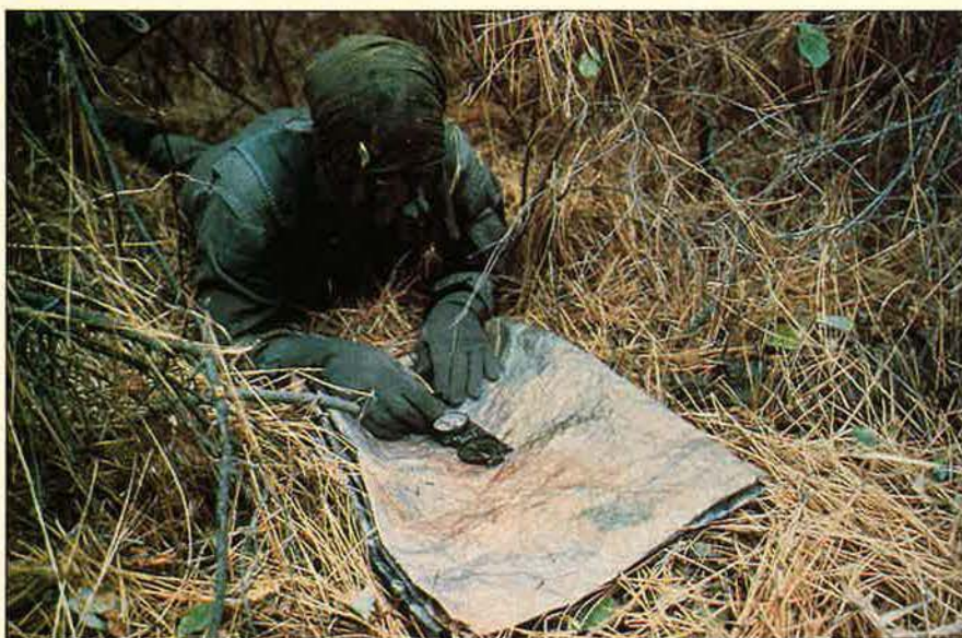
The latest Escape and Evasion chart is much more than a map. It contains information on vegetation, celestial navigation, and first aid. The muted colors serve as camouflage, and because it's made of spun olefin, it's waterproof. The new E&E charts, five years in development, are printed by the Defense Mapping Agency.
