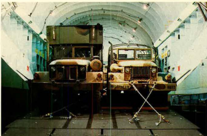
Army vehicles fit comfortably, side by side, in this mockup of the C-17 cargo bay. During the Just Cause operation, eight C-141s were required to deliver eight Sheridan tanks to the drop zone. Four C-17s could have done the job—and dropped other supplies at the same time.
