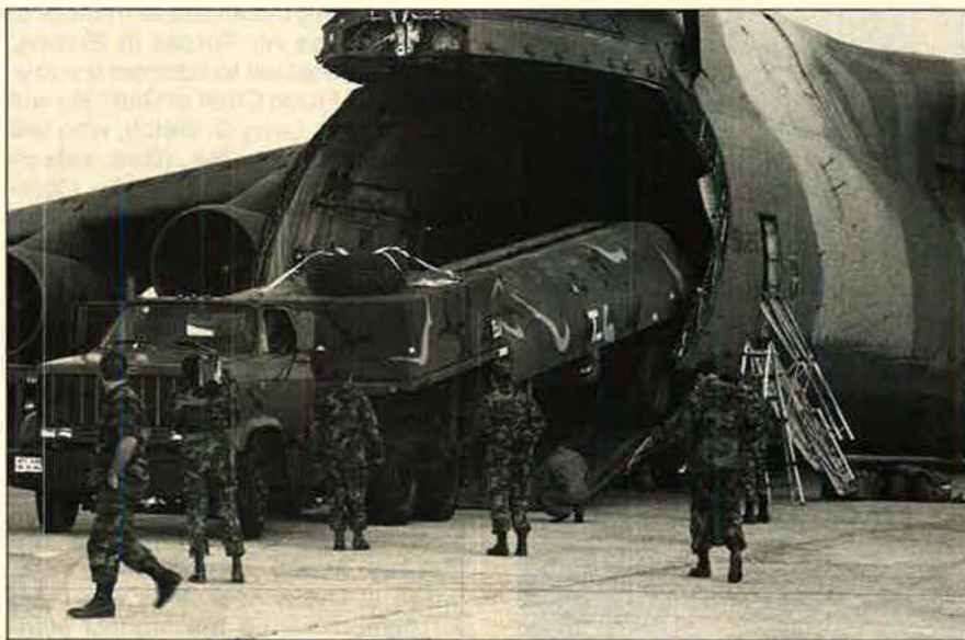
The first 38th Tactical Missile Wing transporter/erector/launcher, with its four BGM-109G ground-launched cruise missiles, is loaded aboard a 60th Military Airlift Wing C-5A on April 11. Twelve other missiles and their TELs were airlifted to Davis-Monthan AFB, Ariz., where they were destroyed under the terms of the INF Treaty.
