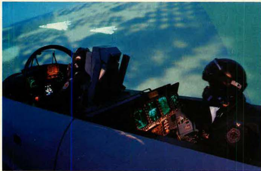
In a far cry from the days of "That Looks About Right," today's F-15E drivers familiarize themselves with the aircraft's many displays in futuristic simulators such as this one. A total of seven cathode ray tubes and the pilot's head-up display give the aircrew vast amounts of data in digestible form.
