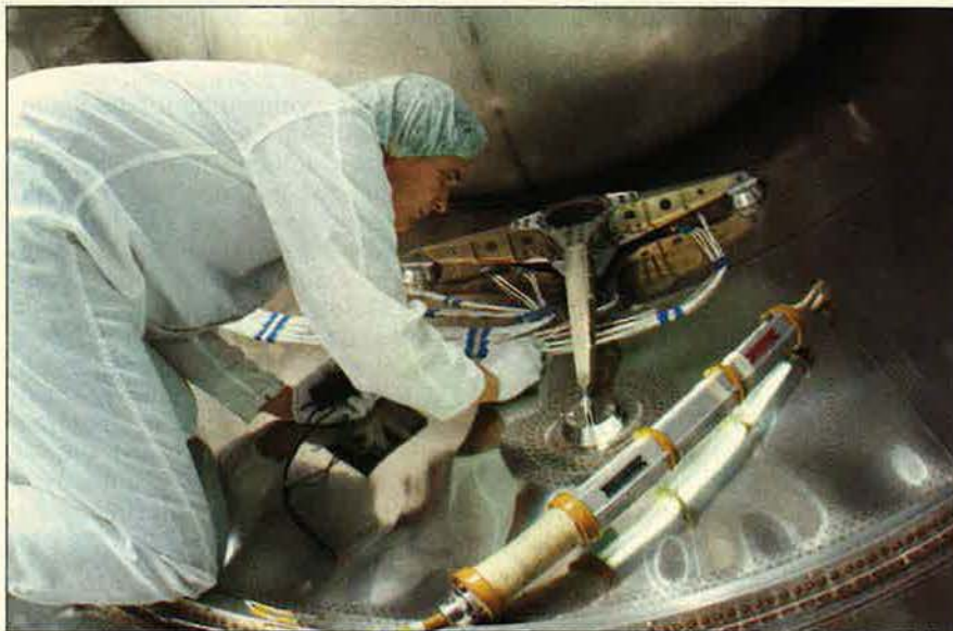
General Dynamics test engineer Rich Fagan inspects strain gauges that measure contraction and expansion of the stainless-steel structure of the Centaur upper-stage space booster. The Centaur, built in San Diego, Calif., is used to boost payloads to geosynchronous orbit after launch from a Titan IV space booster.
