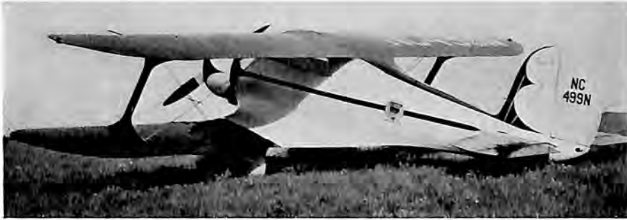
A BEECHCRAFT FOR BUSINESS Model 17-R with Wright Whirlwind engine.
