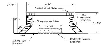
**E12F** — A 12" high, beige color, molded fiberglass, reinforced polyester resin, double shell, prefabricated roof curb with a 3½" cant, corner gussets, 2" thick fiberglass insulation and incorporating a treated 1½" x 3½" treated wood nailer and damper tray.
