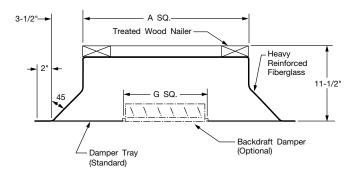
E12 — A 12" high, beige color, molded fiberglass, reinforced polyester resin, single shell, prefabricated roof curb with a 3½" cant, corner gussets and incorporating a treated 1½" x 3½" treated wood nailer and damper tray.
