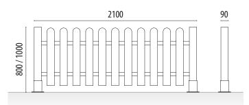
**Fustal model wooden fence** built with autoclave wood.
