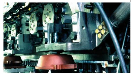
Engine cradle for the high performance Diesel motor made from ADI (model MTU Friedrichshafen Ltd, series BR 8000)
