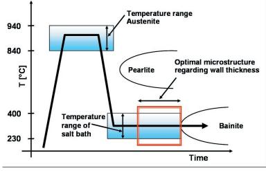
Fig. 3. Schematic of the temperature gradient of the isothermal interstitial transformation
