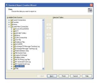
2. Expand the Create New Connection folder in the Data window, and then expand ODBC to open a dialog from which you can select the data source that you want to use - in this case, SAMLTD.
