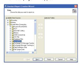
2. Expand the Create New Connection folder in the Data window, and then expand Database Files to open a dialog from which you can search for the datapipe DLL file.
