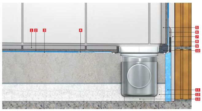
Sectional front view, suggested installations with sound decoupling
